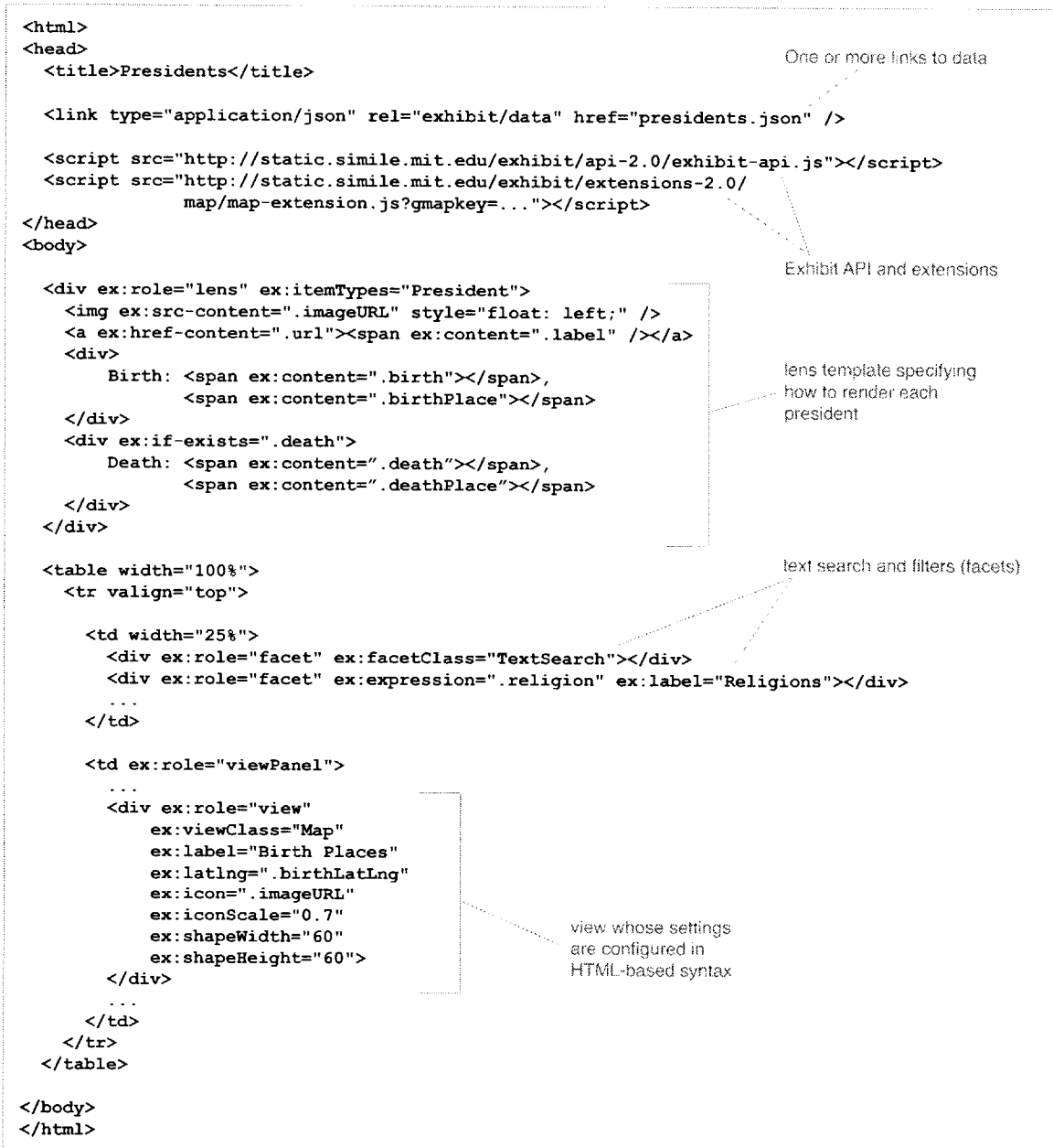
Figure 1.2. An HTML-based syntax is used for configuring the user interface of an Exhibit-powered web page.
