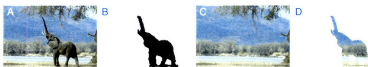
Figure 6-7: Example of “Fragment-Based Image Completion” as found in [41]. [A] original image; [B] region deleted manually; [C] image completed automatically; [D] region that was “made-up” using fragments of the rest of the image.
