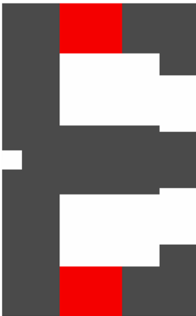
Figure 3.3 Cross sectional view of the MHT-9 magnetic circuit configuration. The permanent magnet is shown in red, and the core material is in grey.
