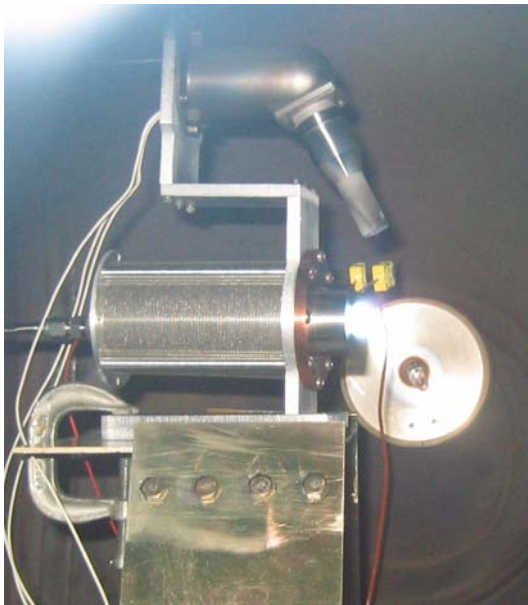
Figure 4.6 The MHT-9 briefly firing during test #1. The plasma is very bright and almost spherical in shape. The large bright circle on the far tank wall is a copper plate reflecting the camera flash. The yellow plastic pieces just above the plasma are thermocouples.
