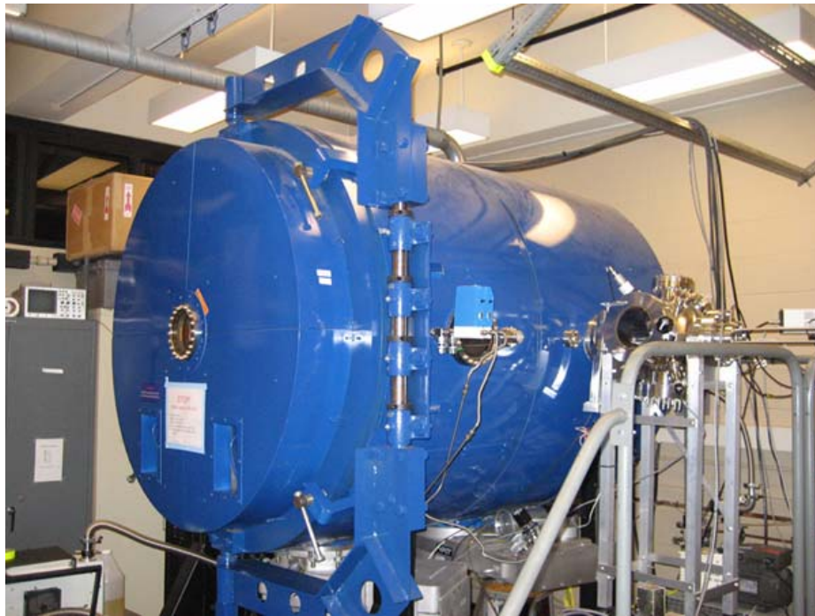
Figure 4.1 The MIT Space Propulsion Laboratory Astrovac vacuum facility.
