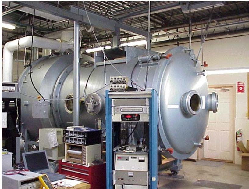
Figure 4.2 The Busek T6 vacuum facility.
