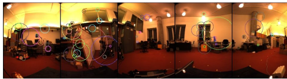
Fig. 1. An omnidirectional camera frame of five outward-looking images. Our camera also collects one upward-looking image (not shown), which is unused by our method.
