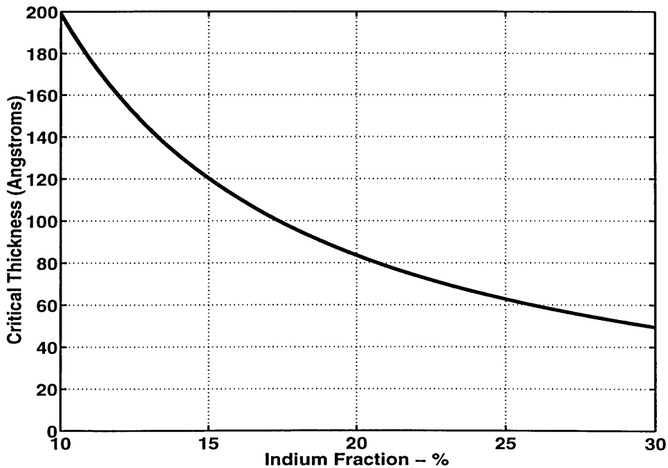
Figure 3.9: Critical thickness for single epitaxial layer of InGaAs on GaAs
