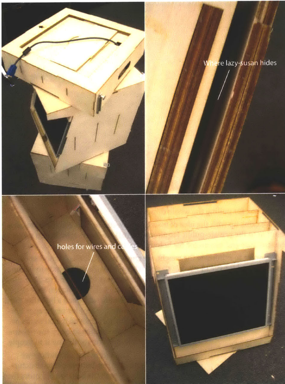
Figure 3.3 Snapshots for the kiosk assembly.
