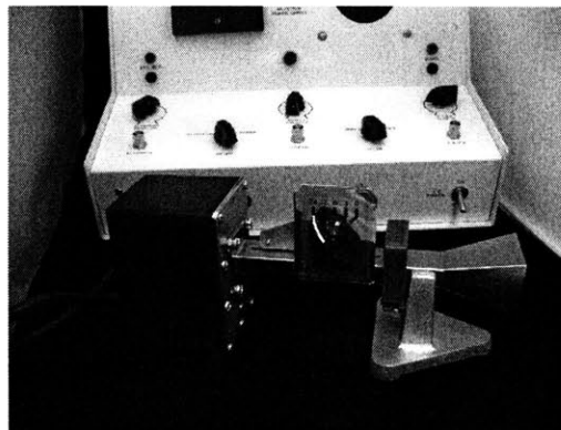
(c) Solid state generator with waveguide
