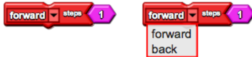
Figure 3-7: A combo box appears over the ‘forward’ label of the block. Users can change this block to a back block, which is in the same family as forward .
