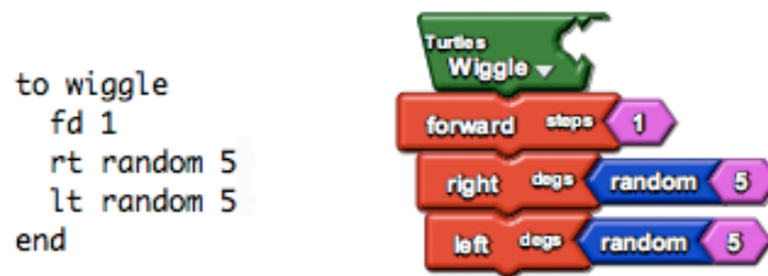
Figure 3-1: The StarLogo and StarLogo TNG code are both expressing the same commands for the procedure wiggle .
