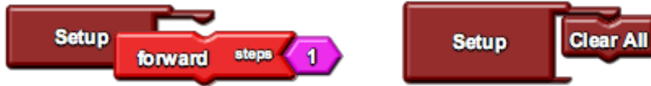
Figure 3-10: Users would try to connect blocks that match the connector shape at the Setup block but find they can not for syntactical reasons even though they visually can.
