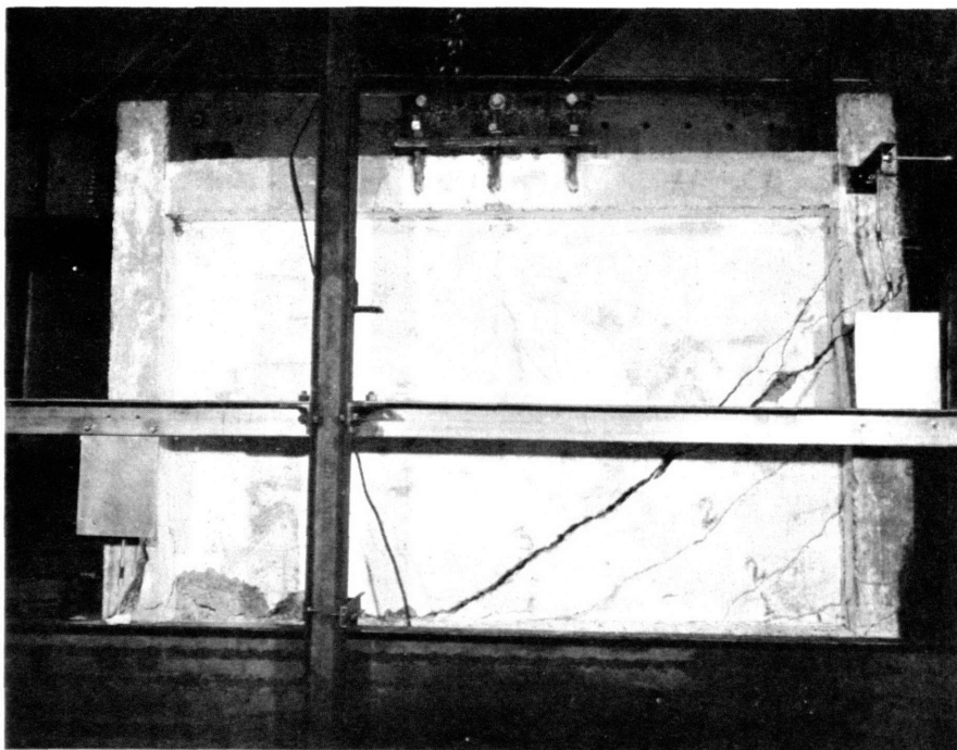
Figure 85 - Crack Pattern of Specimen #4 After Failure of the Connection Between the Reinforcement of the Tension Column and the Support Plate
