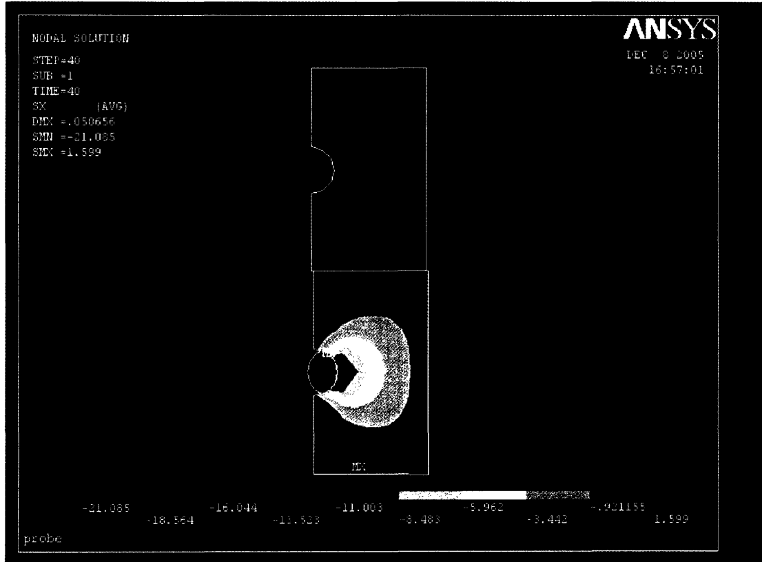
Fig. 22 Close up view of the cable and Incoloy 908 ® rings at step 40 of the analysis. The plot illustrates the transverse stress.
