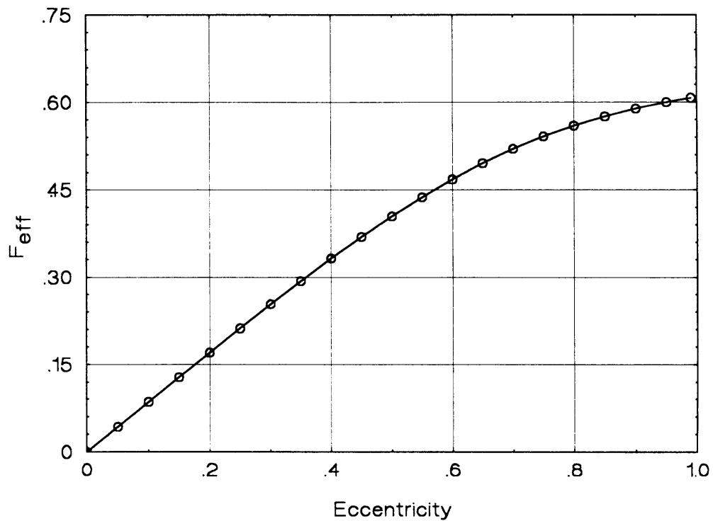
Figure 3.4. Load-carrying efficiency of the 6-pocket, 80 mm diameter FC Bearing #1 of Table 3.1.
