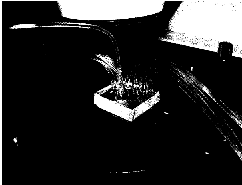
Figure 9 A single microfluidic device with inputs and outputs attached.
