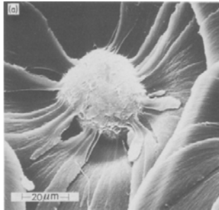
a). a good adherence between matrix and glass beads, using \gamma -aminopropil silan
