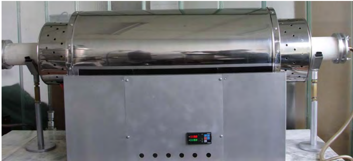
Fig.1. Photo of the setup for deposition of glass carbon coatings.
