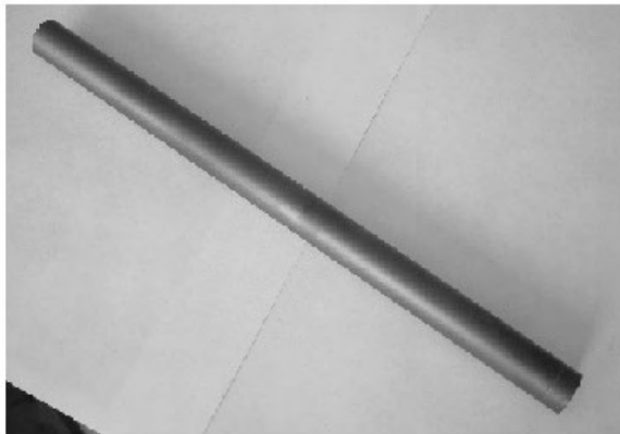
Fig. 7. Shaft – C40 steel; Oxinitrocarburized surface; Exposure at salt fog 96 h; without corrosion
