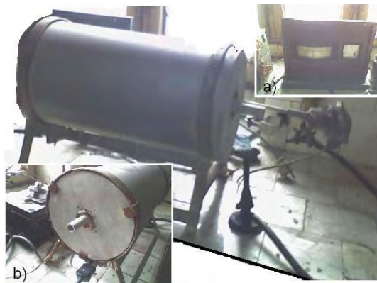
Fig. 8. Experimental installation for pyrolysis graphite revealing as a result of gasifiable model thermal destruction: a) equipment for process parameters control; b) detail of experimental installation.
