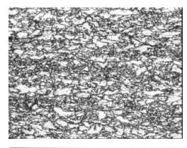
Figure 3. Specimen microstructure with intercritic thermomechanical treatment (table 3) (x 500 magn., Nital etch 2%)
