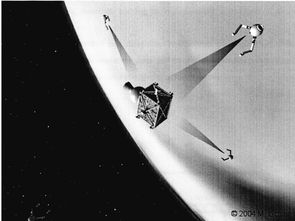
Figure 2.3. Cooperative observation: four sensors distributed about a target object. Image made using OpenGL [68].
