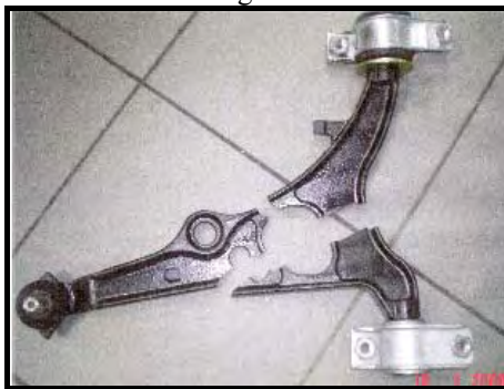
Fig.1. „Arm – wheel support” - cracked piece.
