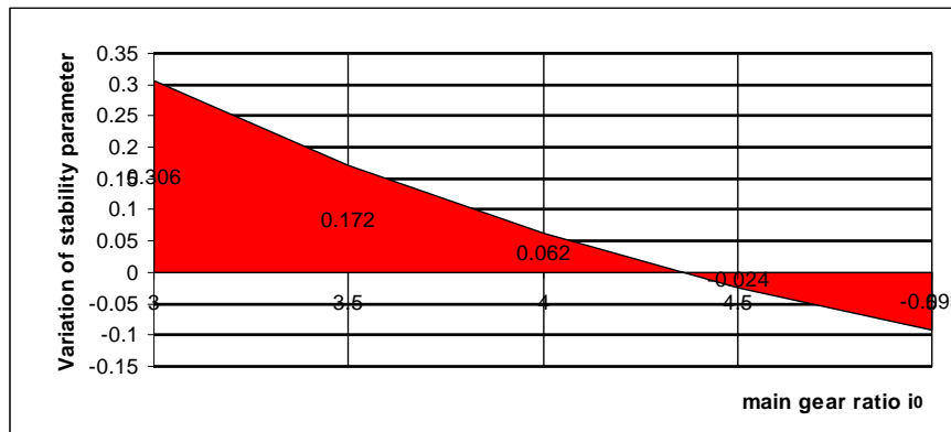
Fig. 13. Variation of stability parameter with main gear ratio change obtained by simulating MATCEL-PROP for propulsion engine power of 64 [kW]
