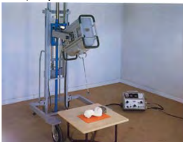
Fig. 6 Portable monoblock type MONOGIL MT 350 / 6 of roentgen ray for research of art objects made of metal, ceramic and stone. Sankt-Peterburg
