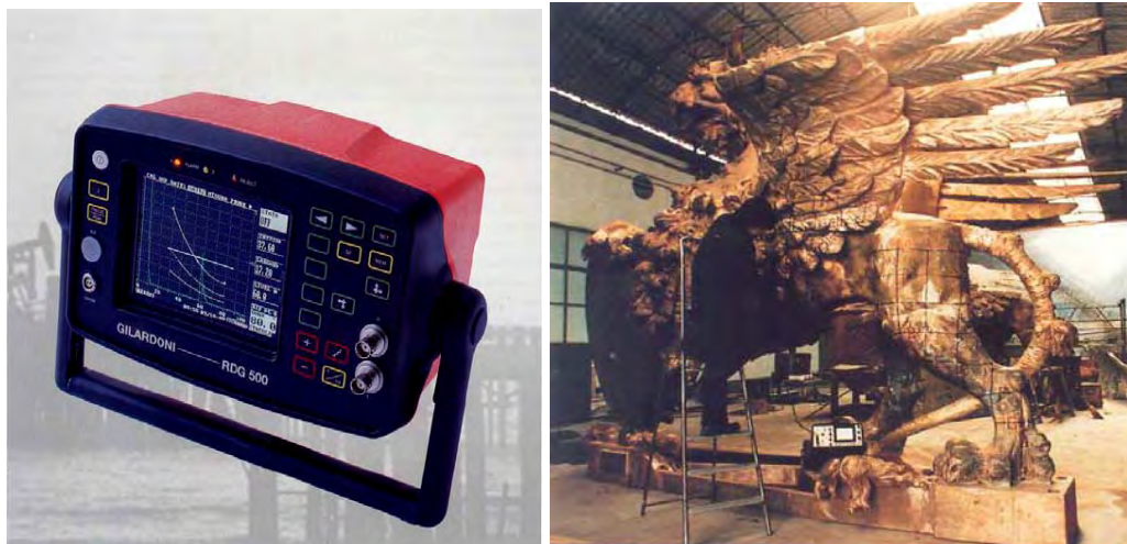
Fig. 8. The defectoscop type RDG 500 to control the layer state of preservation, thickness measurement, detection of hidden defects in metal, ceramic and marble sculptures.
