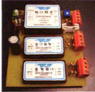
Figure 2-25. Power supply regulation PCB.
