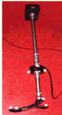
Figure 4-5. Control weight on passive prosthesis with reflective markers and force/torque sensor
