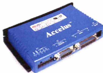
Figure 2-26. Accelus™ digital amplifier from Copley Controls Corp.
