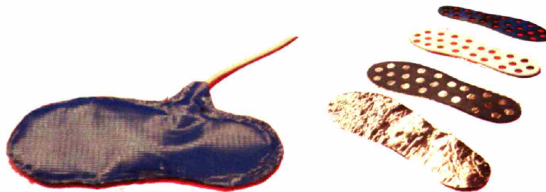
Figure 2-20. Custom made discrete switch insole.
