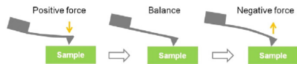
Fig. 9. Schematic of AFM tip/specimen contact under negative and positive applied loads [11]
