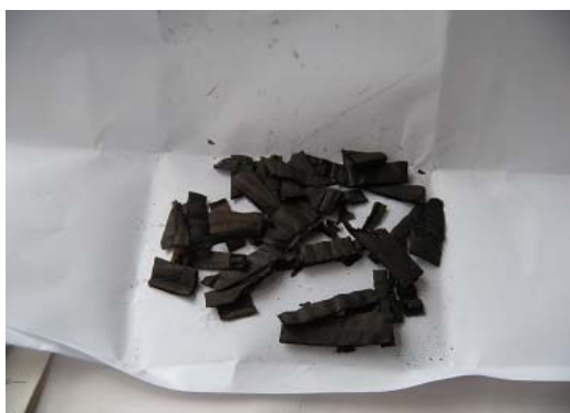
Fig. 4. Solid fraction resulting from pyrolysis process: a – from wood flour, b – from paper.
