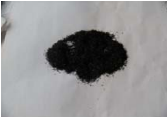
Fig. 4. Solid fraction resulting from pyrolysis process: a – from wood flour, b – from paper.
