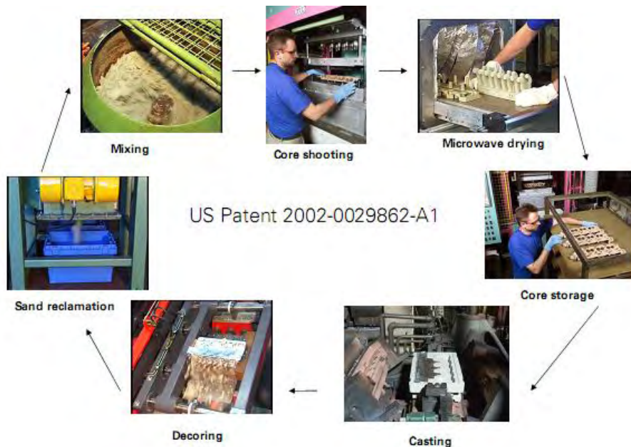
Fig. 1. Castings production using the AWB process.
