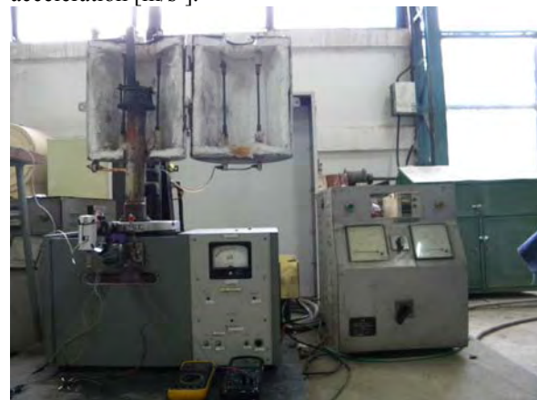
Fig. 2. Plant consists of three heating and vibrating stand for a crucible: 1- vertical furnace with forced bars, 2 - vibrating table, 3 - crucible.
