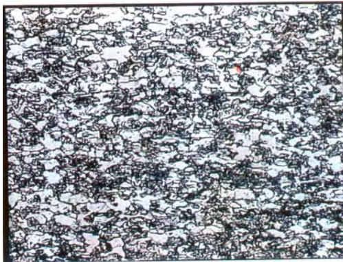
Fig.10. Intercritical thermomechanical treatment state - I variant (x500).
