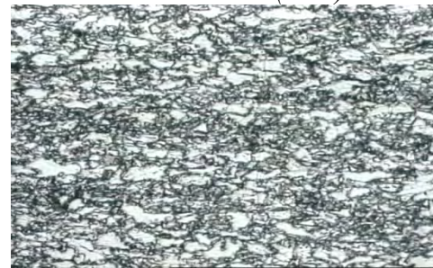
Fig.7. Intercritical thermomechanical treatment state - C variant (x500).
