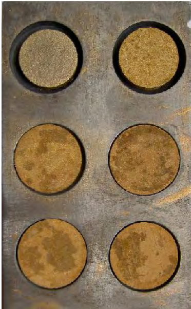
Fig. 2. Bronze powder samples sintered at 750 0 C
