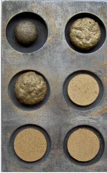
Fig. 1. Bronze powder samples sintered at 850 0 C
