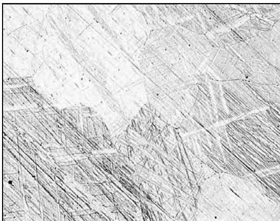
Fig. no. 7 Microstructure of the bath 0 % Ni. (x 100). 1% nital attach. Zn large crystals with macles.
