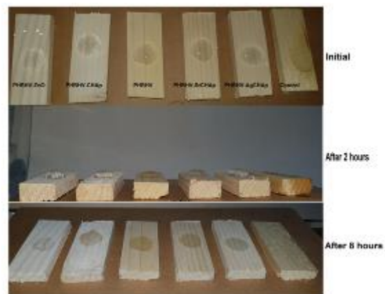
Fig. 7. Water drop absorption at different times
