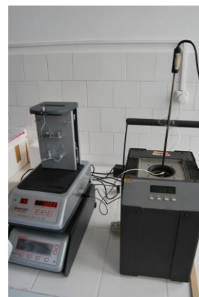
Fig. 7. Calibration thermobalance sensor at 15°, 20° and 30 °C
