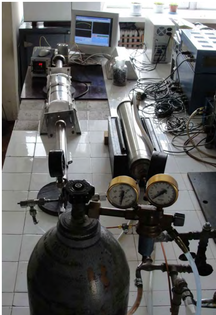
Fig. 1. Installation for producing TiH 2 .
