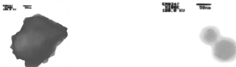
Fig.2. TEM (JEM 1011 / JEOL microscope) micrograph of: uncoated (a) and coated with hydrocarbon (b) powder particles. The coating is seen as a pale halo, with several nanometers thickness, around the particles.
