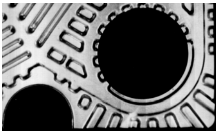
Fig. 5. Uncracked area of the heat exchanger
