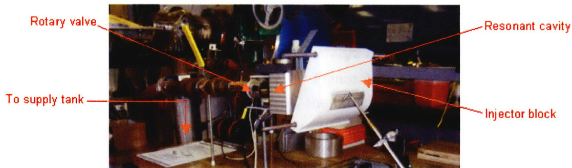
Figure 4-9: The injection setup on test bench
