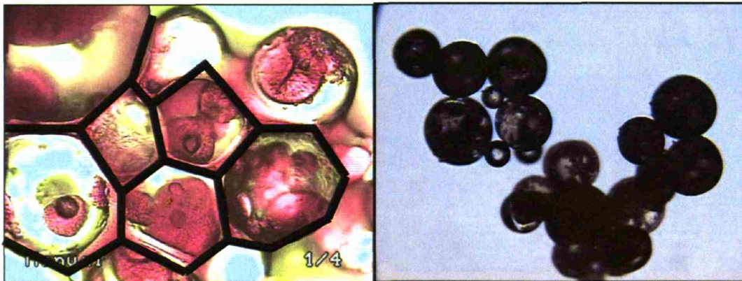
Figure 1-1: Left- Expandable/Deformable PAA-MS in blood deform when juxtaposed and maximize interfacial contact (lines drawn in to highlight surface contact). Right- when microspheres are rigid they interact at small areas which can act as pivots for rolling
