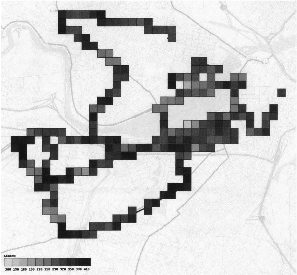
Figure 2-5: Measured coverage map for Boston. Darker squares indicate regions of higher throughput.
