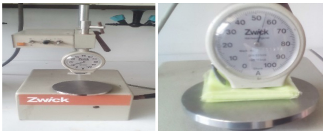
Fig. 4. Hardness tester at Polymer laboratory IAP.
