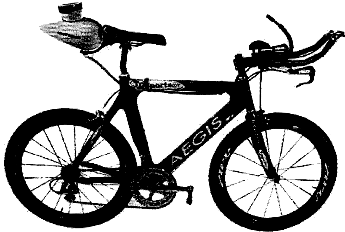
Figure 11: The NeverReach system ($99) mounts behind the seat and offers easy on-the-fly refill capability and a huge 1890 mL (64 oz.) container.
