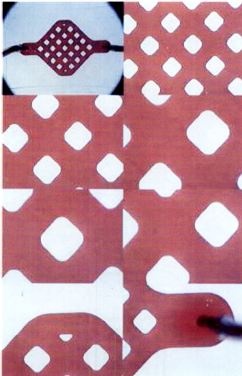
Figure 5. 11 Photos of microfluidic device taken after 7 hours of blood perfusion. The possibility of thrombus formation was studied by microscopy at following a 6 hour perfusion at a constant flow rate of 0.250 \text{ ml min}^{-1} . Images are displayed at various locations in the microchip at approximate magnifications ranging from 5-10X. Images are displayed immediately following the perfusion period. No thrombus was observed at any point of the device. The width of single channels is 1.197 mm.
