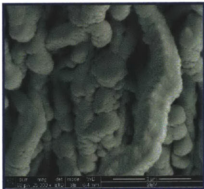
Figure 5-9: CNT side-wall coverage after different durations of metal sputtering.
