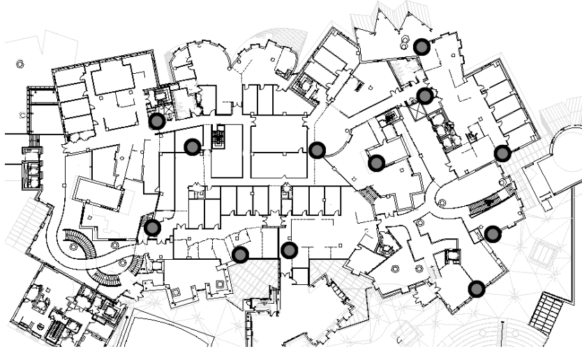
Figure 4-1: One Floor of our Testbed. Nodes' location on one floor of our 3-floor testbed.
