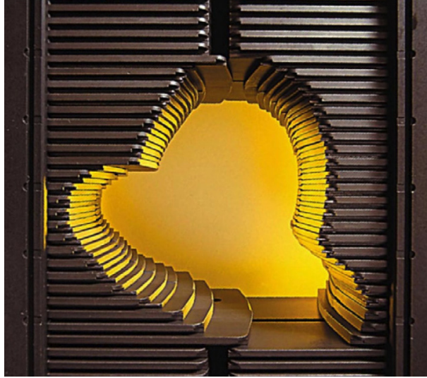
Figure 4-13: A beam's eye-view of the multi-leaf collimators used for beam modulation in IMRT. The radiation beam passes through the gap made by multiple layers of collimators. By sliding the collimators, the shape of the gap is changed. Consequently, the distribution of the radiation dosage introduced to the body can be controlled. Credits to: Varian Medical Systems, http:// www.varian.com , April 15, 2007.
