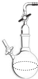
Figure 23. Schlenk flask with a flow control adapter used to store stock solutions of Mo bispyrrolide complexes, chiral diols, and substrates.
