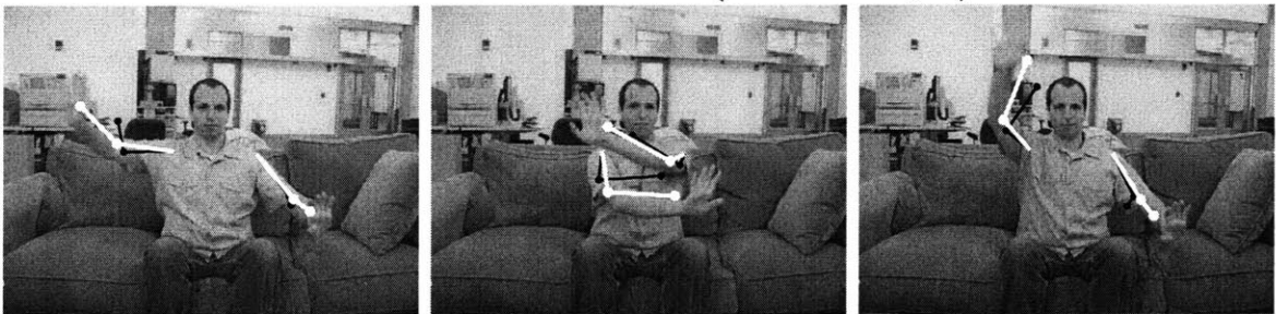
Figure 4-10: (top) Twelve frames were annotated with the joint positions of the subject in a 1500 frame video sequence. (middle) The recovered positions of the hands and elbows for the unlabeled frames are plotted in white. The output of fully-supervised nonlinear regression using only the 12 labeled frames and no unlabeled frames is plotted in black. Using unlabeled data improves tracking significantly. (bottom) Recovered joint positions for frames that were not in the training set. The resulting mapping generalizes to as-yet unseen images.
