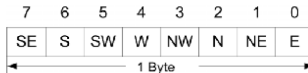
FIGURE 3.13 THE FORMAT OF DIRECTION INDICATOR BYTE (DIB), EACH BIT IS USED TO REPRESENT ONE DIRECTION
