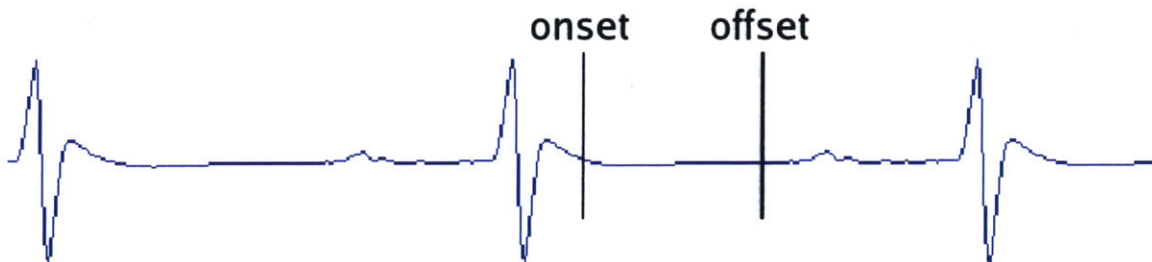
Figure 2-20: The repolarization segment onset point is the point 1 ms beyond the J point (which wqrs often inaccurately detects as occurring at the J peak, as discussed in a previous section); the offset point is the point 40 percent of the RR interval beyond the onset point. That is, if the RR interval is 10 ms and the J point occurs 0.6 ms after the R peak, then the repolarization segment onset is determined to be 1.6ms after the R peak (1 ms beyond the J point) and the offset is determined to be 5.6ms after the R peak (4.0 ms, or 40 percent of RR interval, after the onset). The calculation is performed on a template comprised of a trailing 64-beat point-by-point average after cubic spline baseline removal, as described in chapter 6.
