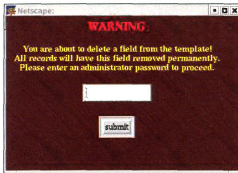
Figure 4-6: The user is attempting to delete a database field, which not only affects the record template but also removes this corresponding field from the back-end SQL database. Such a drastic action should be verified! The user is required to enter an administrator password to proceed.
