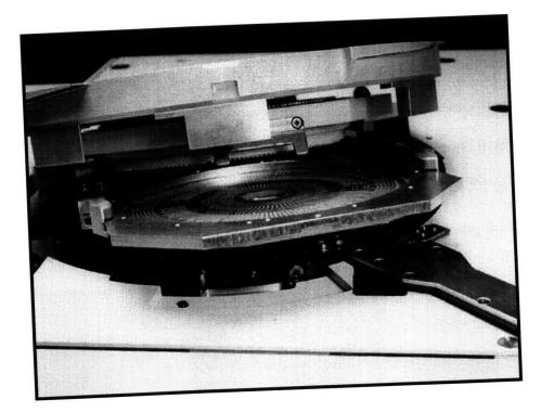
Figure 1.11: Photograph of a Typical Testhead/Prober Interface
