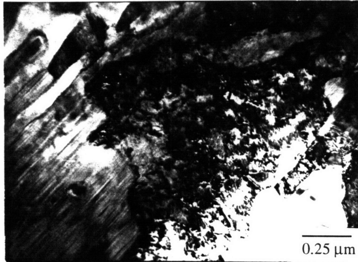
Figure 5.19 TEM of the compressed Ti-80 Cr alloy annealed at 1000°C.
