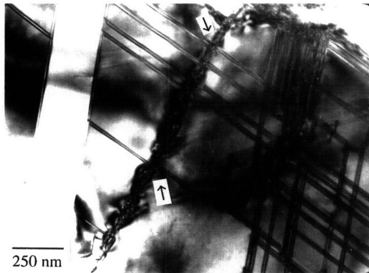
Figure 5.18 Faults displaced about 20 nm across the shear band in the deformed \text{TiCr}_2 .
