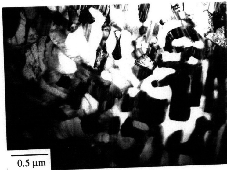
Figure 4.26 The \text{TiCr}_2 Laves phase in the Ti-80 Cr alloy annealed at 1000^\circ\text{C} is interconnected.
