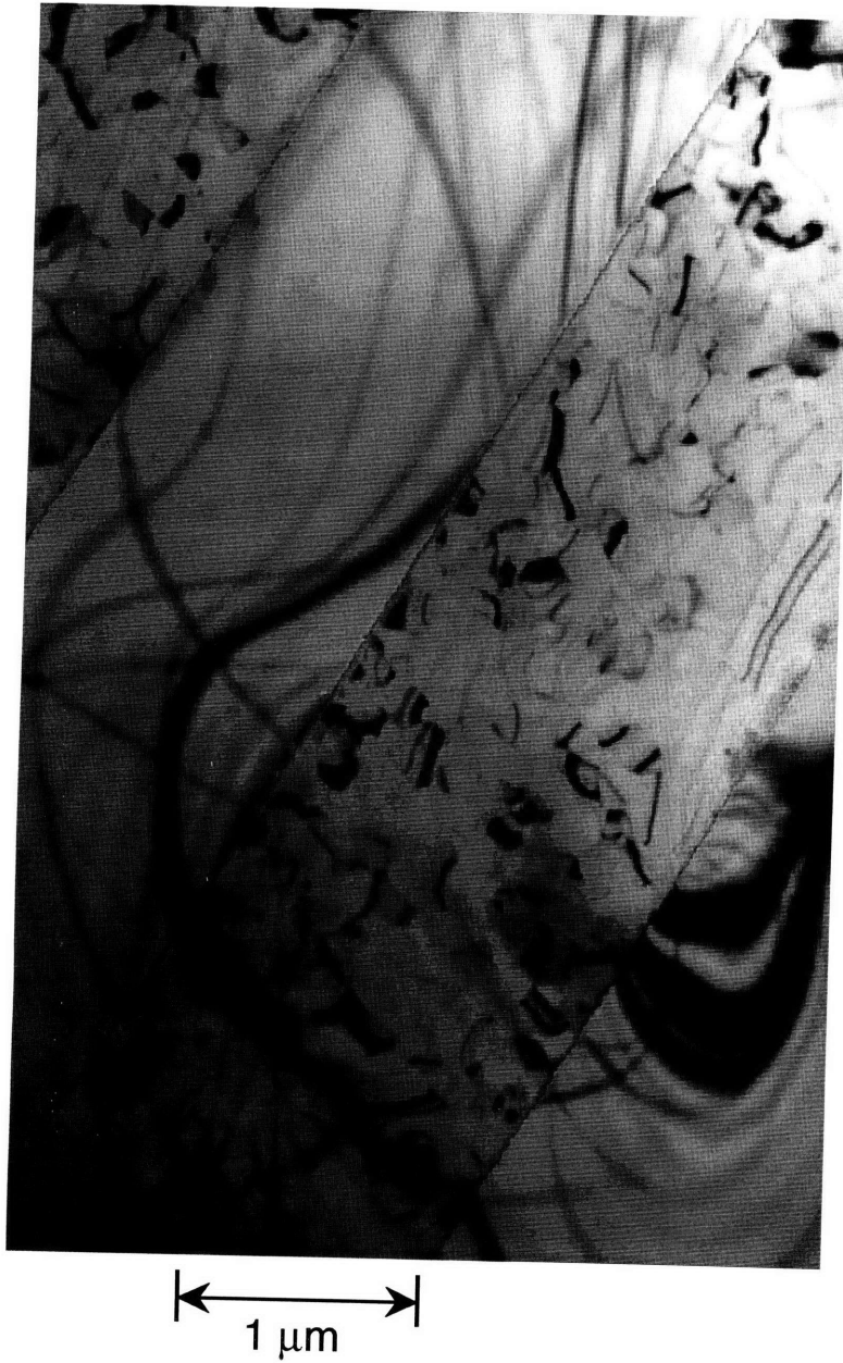
Fig. 4.2.1.2. A TEM picture of an Al/Cu IDT finger. Post-burn-in.
